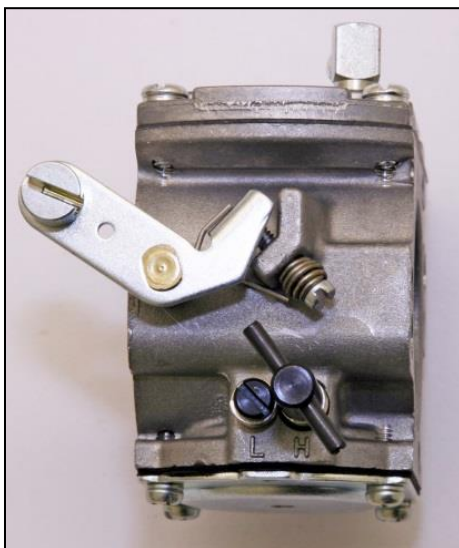
Picture of the Carb Low Jet, High Jet & Tick over Adjustment Screw
