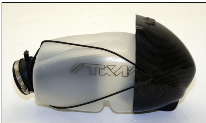
Picture of the Optional Wet Cover Fitted to Air Induction box
