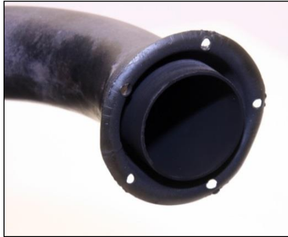
Picture of Inside of Exhaust Bend Manifold for Carburation Checking
