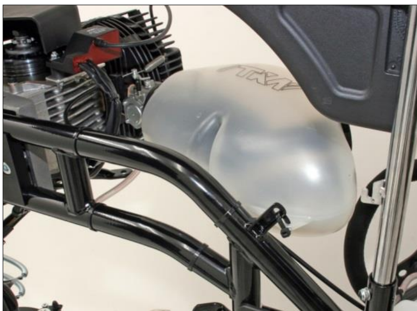
Picture of Air Induction Box Cable Tied to Frame
