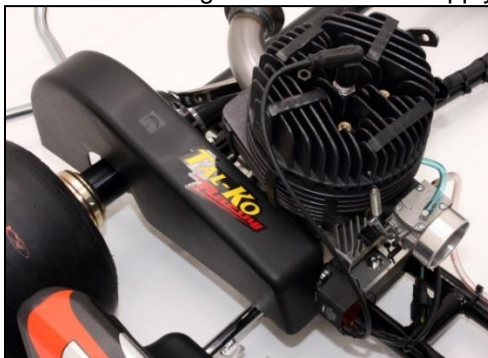
Picture of Fully Enclosed Guard Covering Clutch as well as Chain
