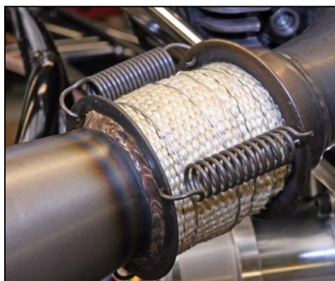
Picture of TAG Exhaust Flex with Wired Wrap
