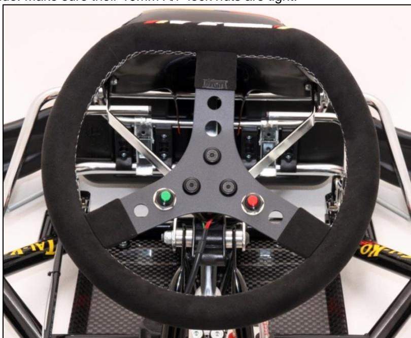
Picture of Start Stop Buttons fitted to Steering Wheel
