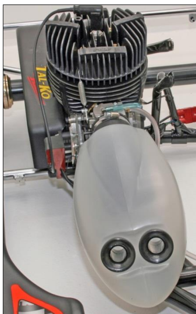
Picture of Air Induction Box Fitted
