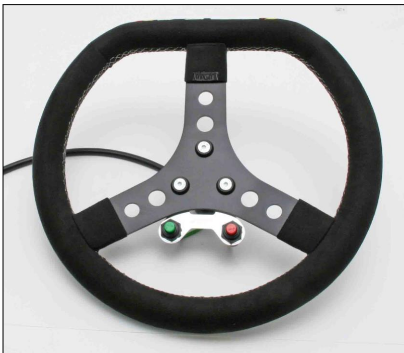
Picture of Start Stop Buttons in Tal-Ko supplied steel chrome bracket
