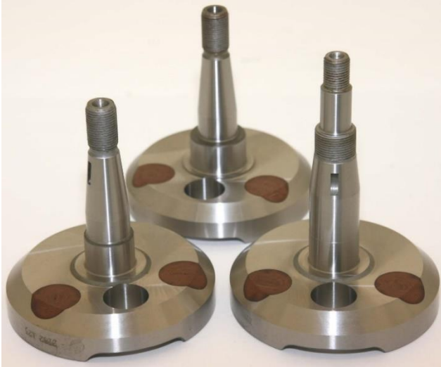
Old style Direct Drive with 20mm Bearing New style Direct Drive with 25mm Bearing Old style Horstman with 20mm Bearing
